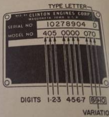
Fig. CL2—Typical nameplate from Clinton engine after model identification system changed in late 1961. First seven digits indicate basic features of engine. Engines with "Mylar" (plastic) nameplate have engine type and serial numbers stamped on the cylinder deflector next to the nameplate.
